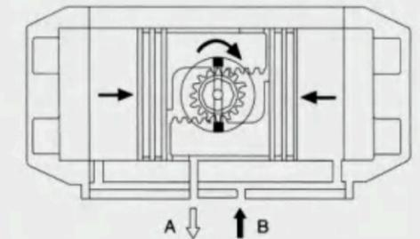
Input the air into Port B forces the pistons move inwards, the pinion turns clockwise and close the valve, then the air be exhausted from Port A.
