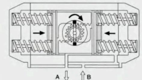
When loss air pressure or power, the stored energy in the springs forces the pistons inwards, causing the pinion turns clockwise while air be exhausted from Port A.
